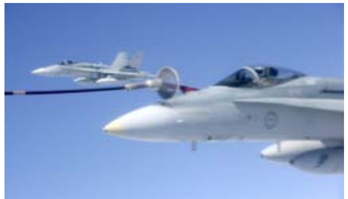
F/A 18 air refueling with probe and drogue system Photo RAAF
