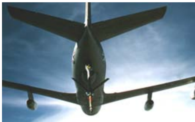
The KC135 boom at the pre-contact position
