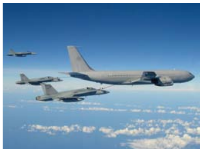
Two F/A 18 aircraft receive fuel from a RAAF B707 Photo RAAF
