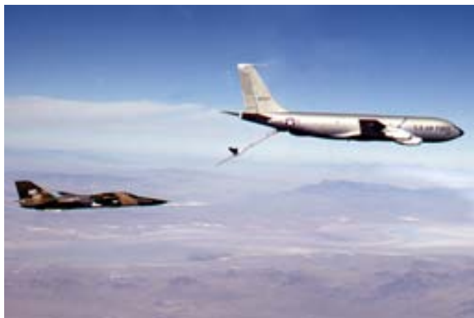
RAAF Crew in USAF F111A before refuelling from a KC135. Photos Lance Halvorson
